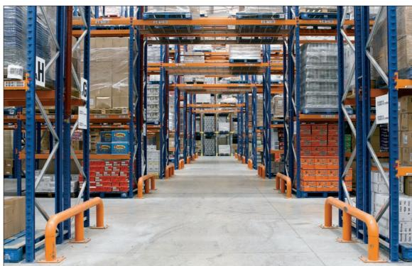
**Above:** Drive-in racking incorporates bespoke modifications with sprinkler protection
